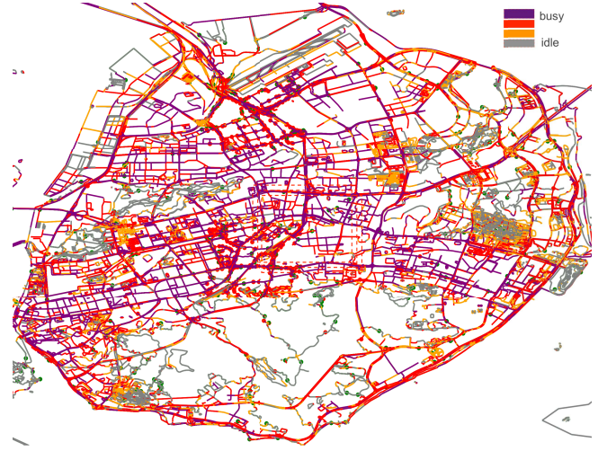
Fig. 4. The map of taxi trajectory coverage in Xiamen City based on the Xiamen Taxi Dataset. The color of each road segment is determined by the number of times covered by taxis.
