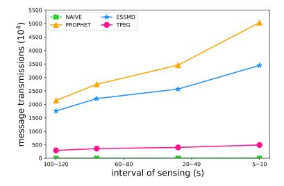
Figure 11. Impact of sensing interval on the number of message transmissions.
