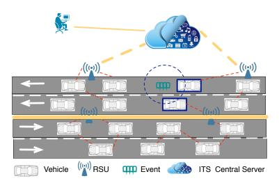
**Figure 1.** Illustration of a vehicular sensing system. Nodes generate pieces of data and send them to fog nodes (RSUs). RSUs provide computation, storage and networking services between the vehicular nodes and ITS cloud.
