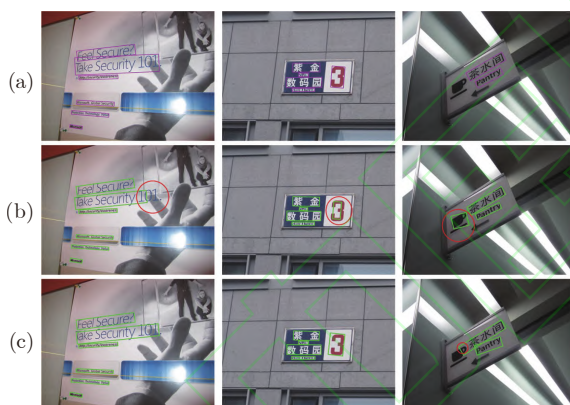
图 5 SDET 与基线模型的检测结果对比: (a) 真实标签; (b) 基线模型检测结果; (c) SDET 训练后的模型检测结果 Fig.5 Comparison of detection results between SDET and baseline models: (a) ground-truth; (b) detection results of baseline models; (c) detection results of models trained with SDET
